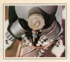
U.S. M3 infrared sniperscope from rear. Knob on left (A) controls electronic focusing of telescope while knob on right (B) allows varying intensity of reticle; consists of small vertical bar of light that appears in field of view. Can be turned off for surveillance and, via rheostat, made progressively brighter for actual sniping work. Center cable (with blue connector) provides power to operate 30-watt IR light
